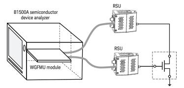
Figure 3. A single B1500A WGFMU module can comprise an RTS noise measurement system
