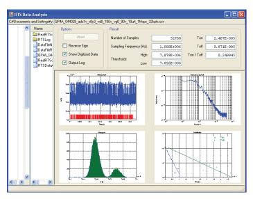
Figure 4. Sample program to analyze RTS noise properties
