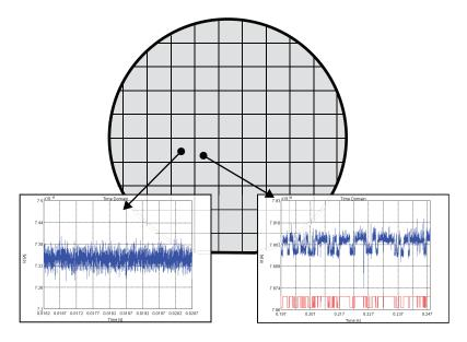
Figure 9. Plot showing variations in RTS noise across a wafer
