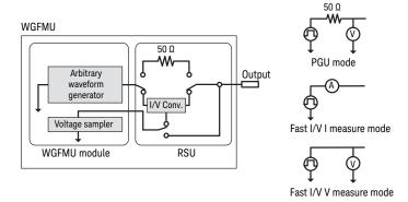
Figure 5. Simplified circuit diagram of the WGFMU module
