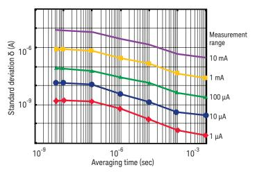
Figure 7. Noise reduction of measured current as a function of averaging
